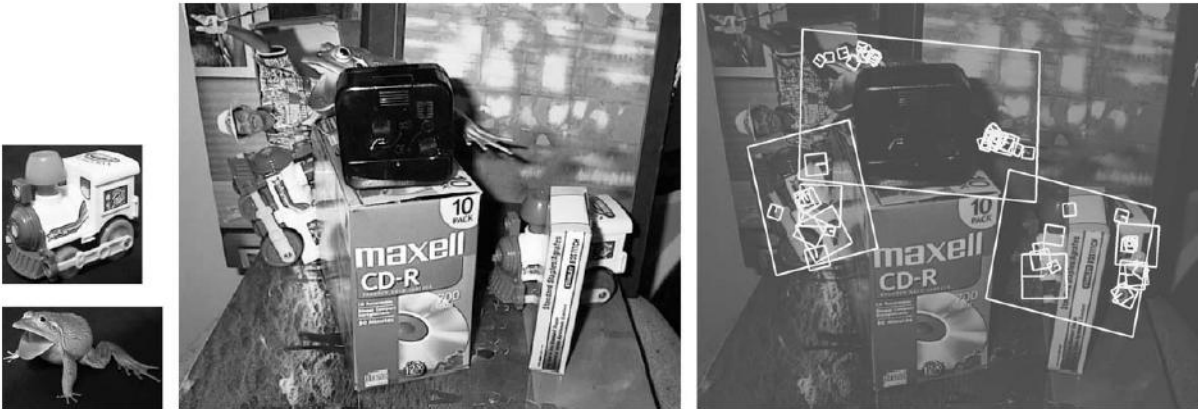
Figure 3. Identification of the 2 training objects on the left in a cluttered image with high occlusion, using SIFT [1]
