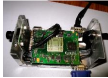
a home-made PCB that includes a Virtex4 and some quite large bandwidth to/from QDR memories
