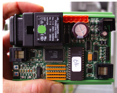
Fig. 6. The floor tile slave controller board.
