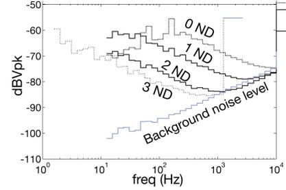
**Fig. 8** Octave band noise spectra of  $V_p$  for various background illumination levels. The number  $X$  of decade neutral density filters is  $X$  ND. The vertical scale is power/octave; it rises for the background flat noise spectrum.
