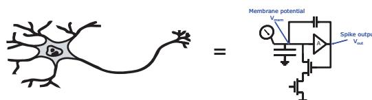
Local analog computations (e.g. I&F neurons) are performed by time-continuous analog transistor circuits integrated in large arrays
