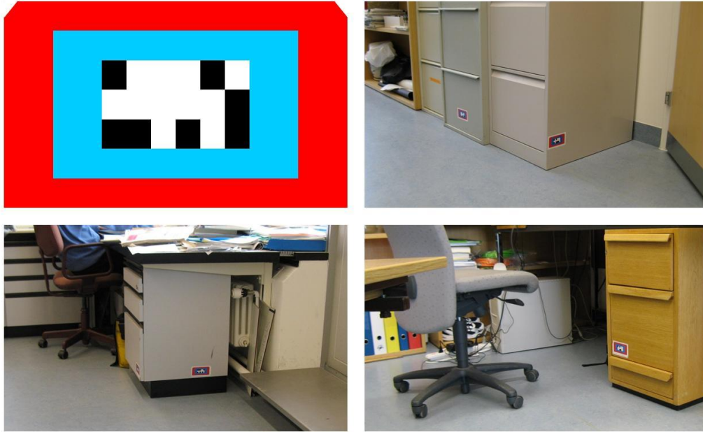
Figure 17: Top left panel: a “landmark” sticker, original size 90x45mm, with easy-to-detect red-blue outside boarder and binary-coded identity inside. Remaining panels: examples of objects labeled by landmarks, which all have a large area of unique color.
