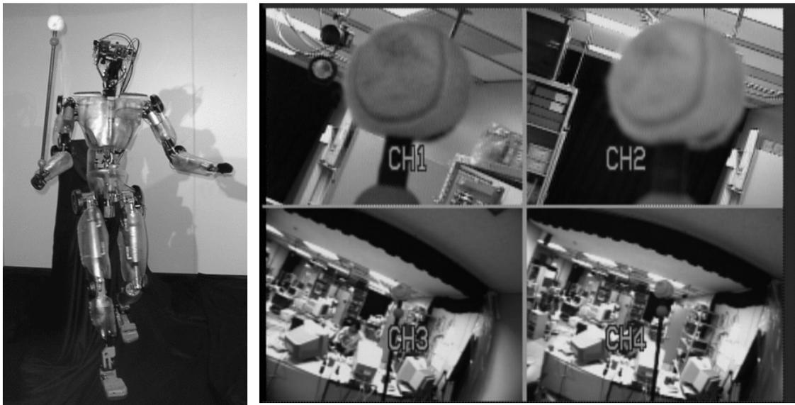
Figure 2: (left) The humanoid robot performing the task of pole-balancing; (right) monitor output of all four cameras (upper: foveal vision, lower: peripheral vision)
