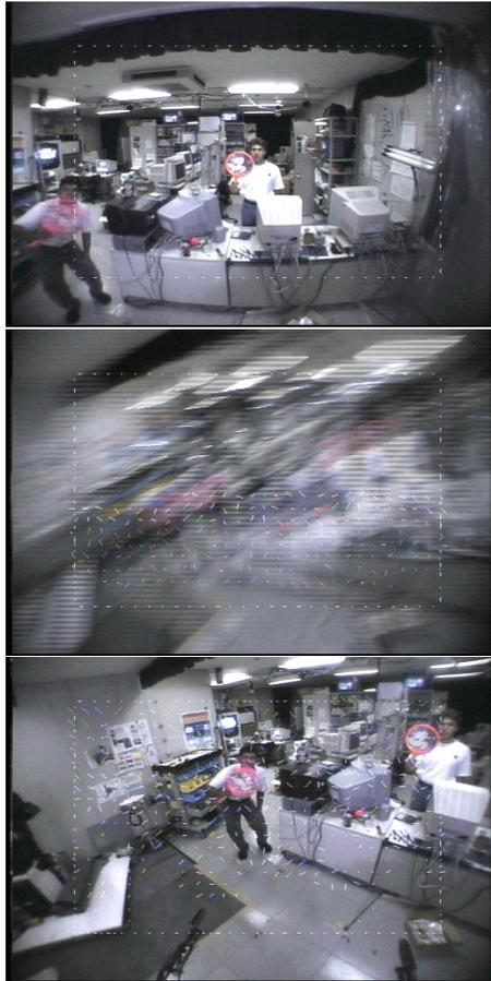
Figure 12: Snap shots of the robot's peripheral view before, during, and after an attentional head-eye saccade, taken at 30 Hz sampling rate. Superimposed on the images is the visual flow field.
